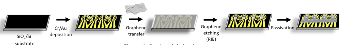
Figure 1: Devices fabrication process.
